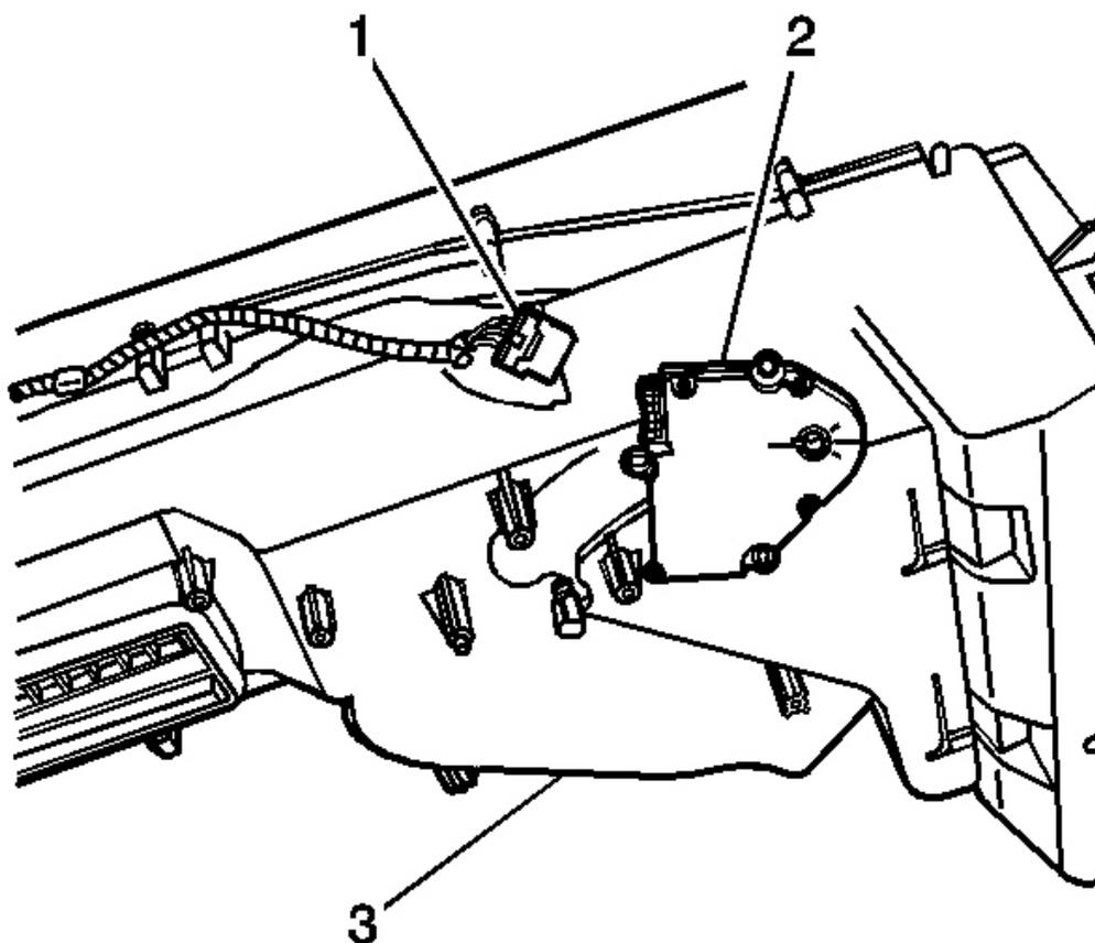
**Fig. 23: Left Air Temperature Actuator & HVAC Module Assembly**
