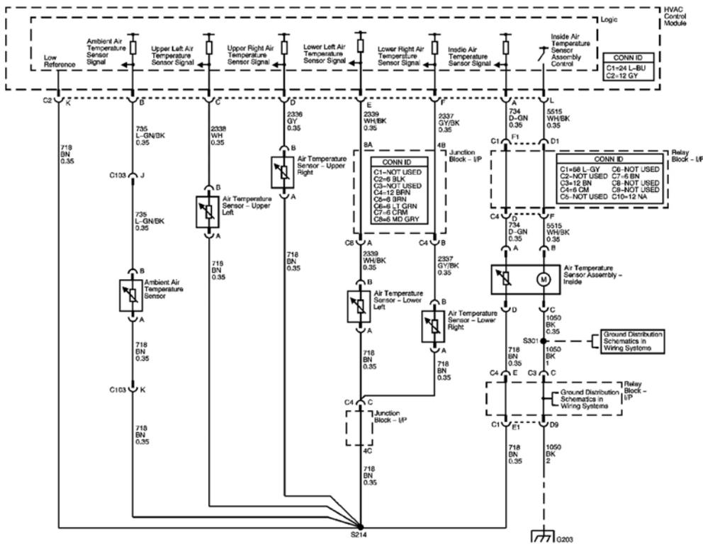
**Fig. 4: Air Temperature Sensors Schematics**
