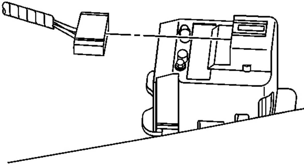
**Fig. 38: Electrical Connector & Inside Air Temperature Sensor**
