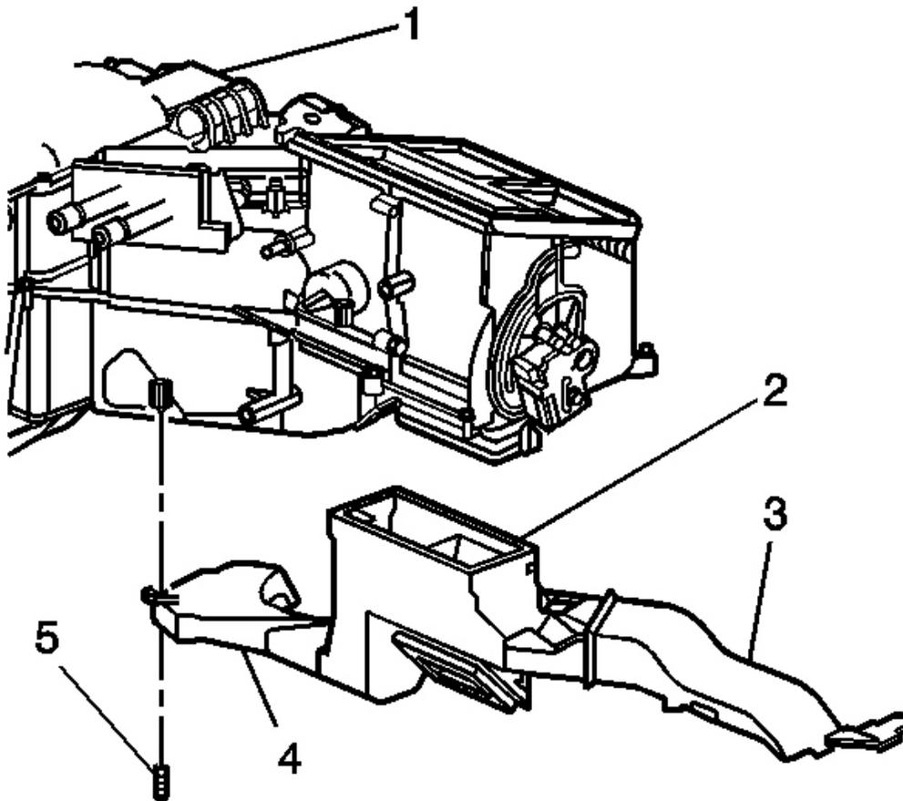
**Fig. 17: Floor Air Outlet Duct**
