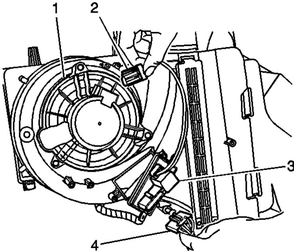
**Fig. 14: Blower Motor Control Processor & HVAC Module Assembly**
