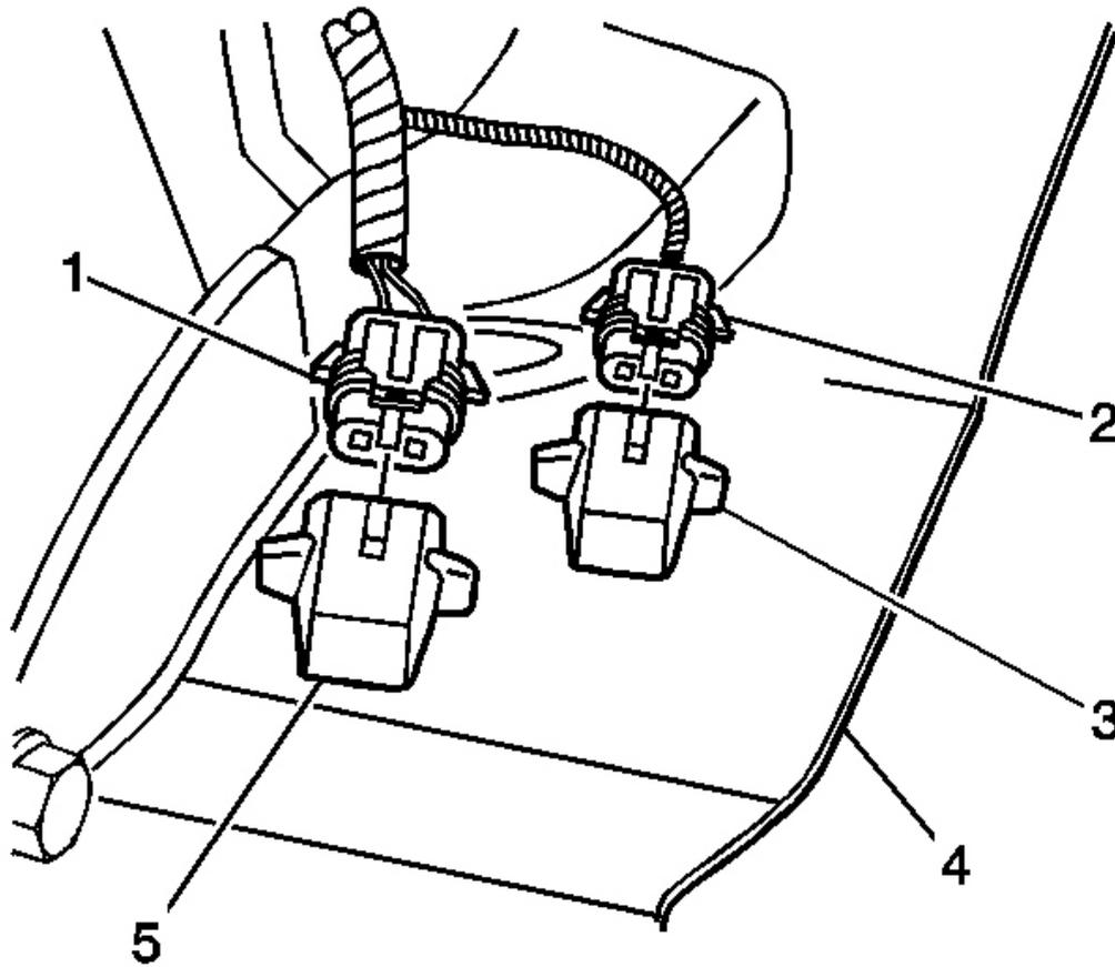
**Fig. 33: Ambient Air Temperature Sensor**
