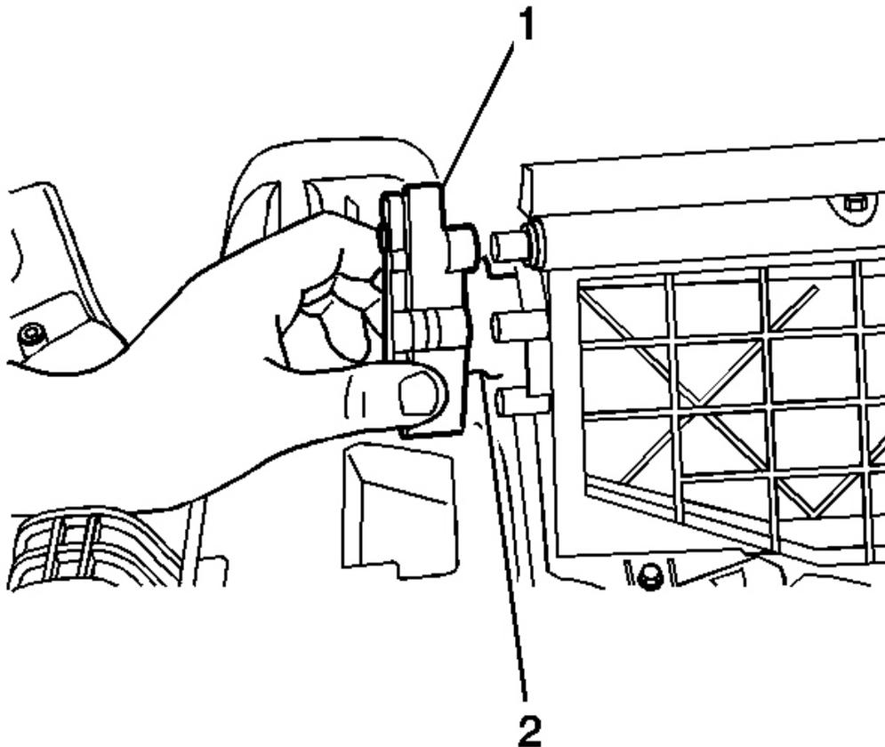
**Fig. 15: Recirculation Actuator & Recirculation Housing (Visteon)**
