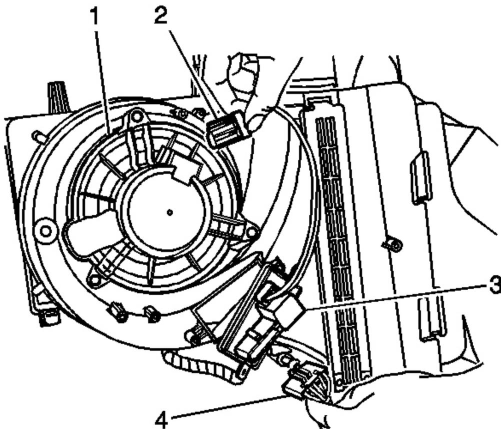
**Fig. 13: Blower Motor Control Processor & HVAC Module Assembly**
