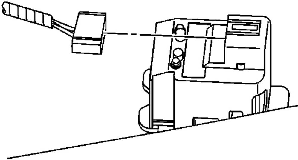
**Fig. 35: Electrical Connector & Inside Air Temperature Sensor**
