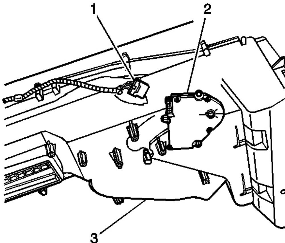
**Fig. 24: Left Air Temperature Actuator & HVAC Module Assembly**
