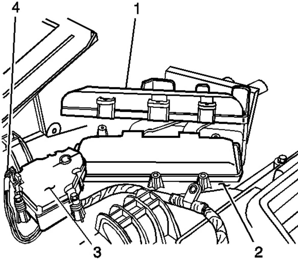
**Fig. 21: Right Air Temperature Actuator & HVAC Module Assembly (Visteon)**
