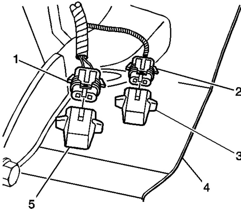
**Fig. 34: Ambient Air Temperature Sensor**
