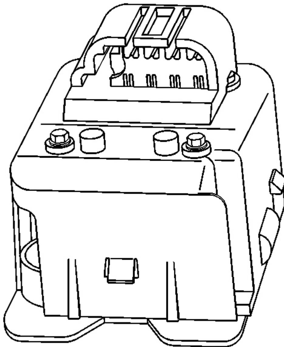
**Fig. 37: Inside Air Temperature Sensor & Headliner**
