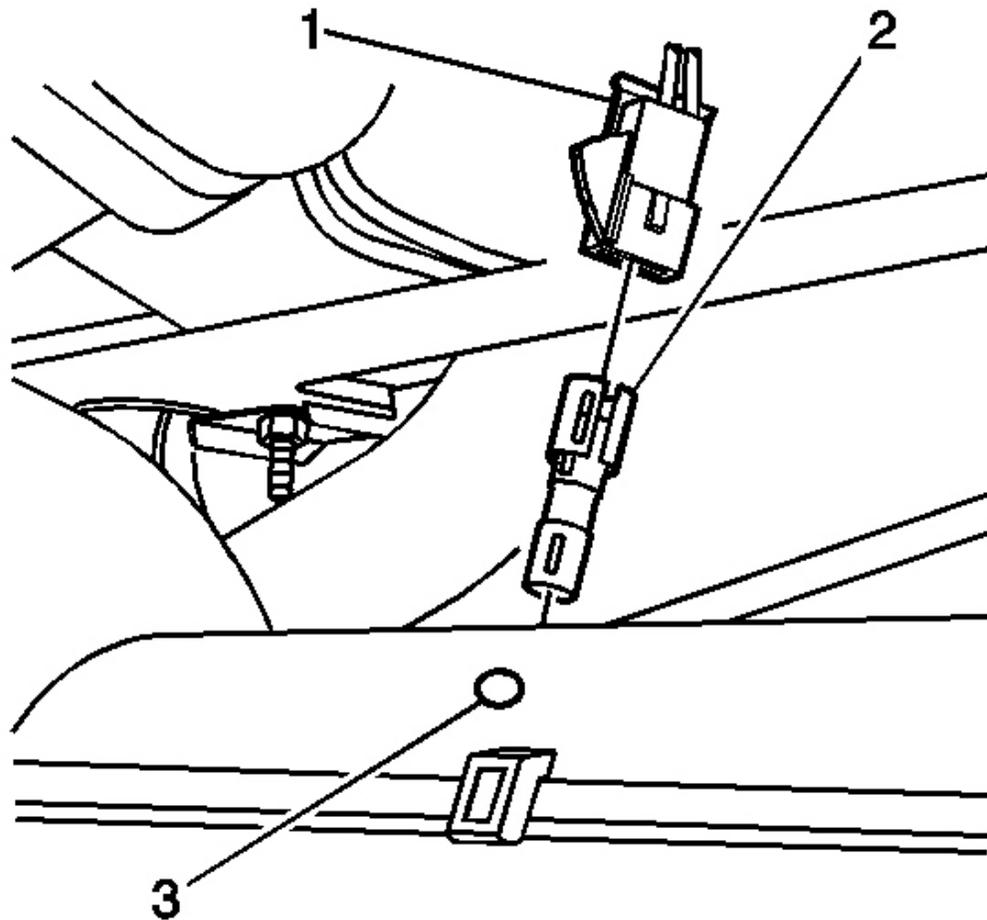
**Fig. 26: Upper Right Air Temperature Sensor & Air Distributor Duct**
