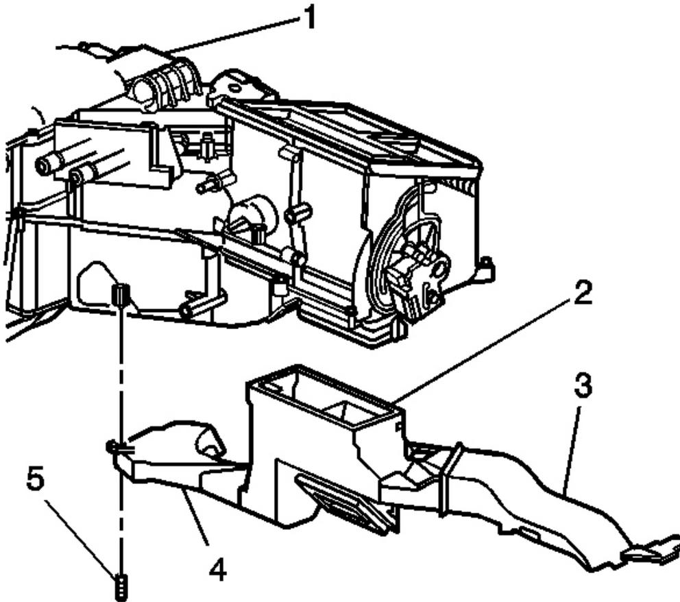
**Fig. 20: Floor Air Outlet Duct**
