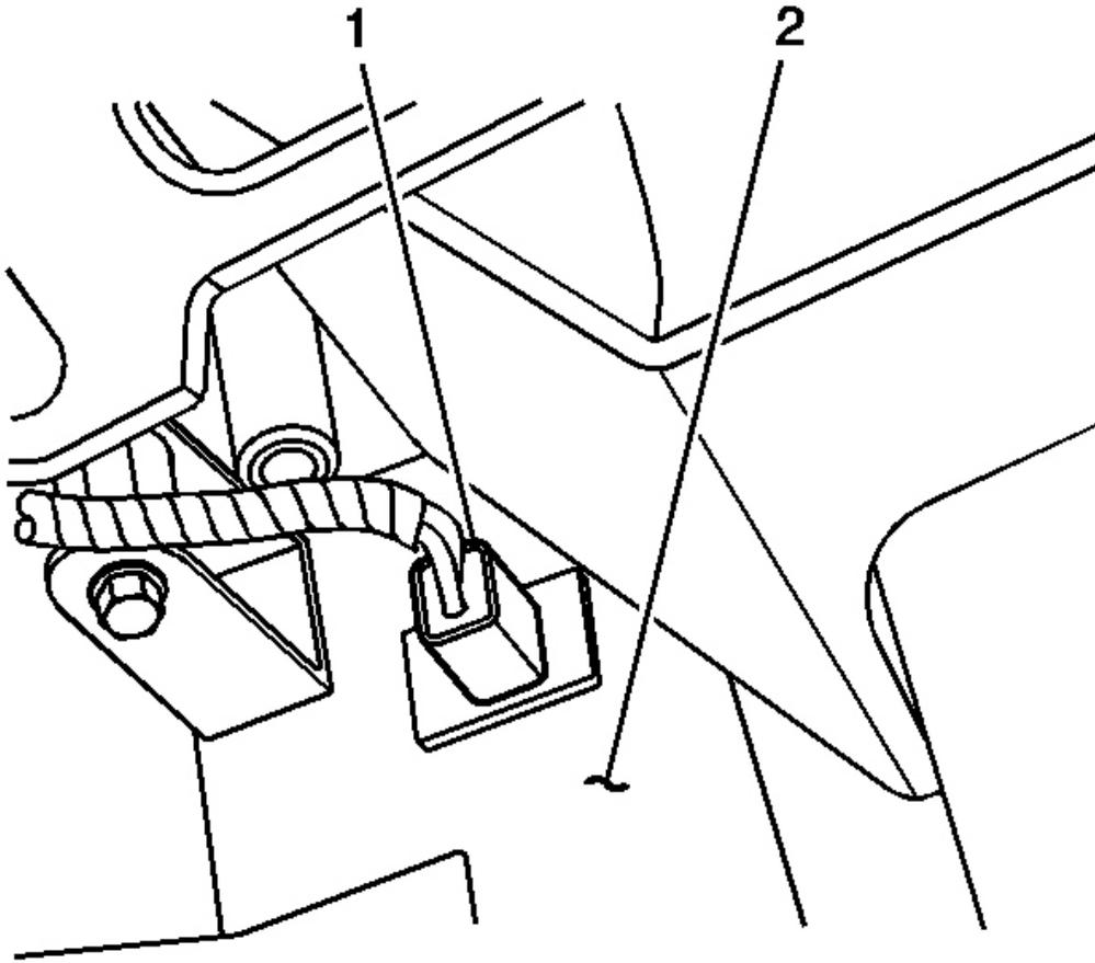
**Fig. 31: Lower Right Air Temperature Sensor**
