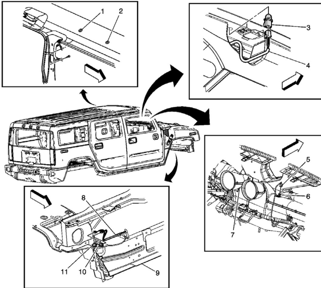
**Fig. 8: HVAC Subsystem Component Views (1 of 2)**
