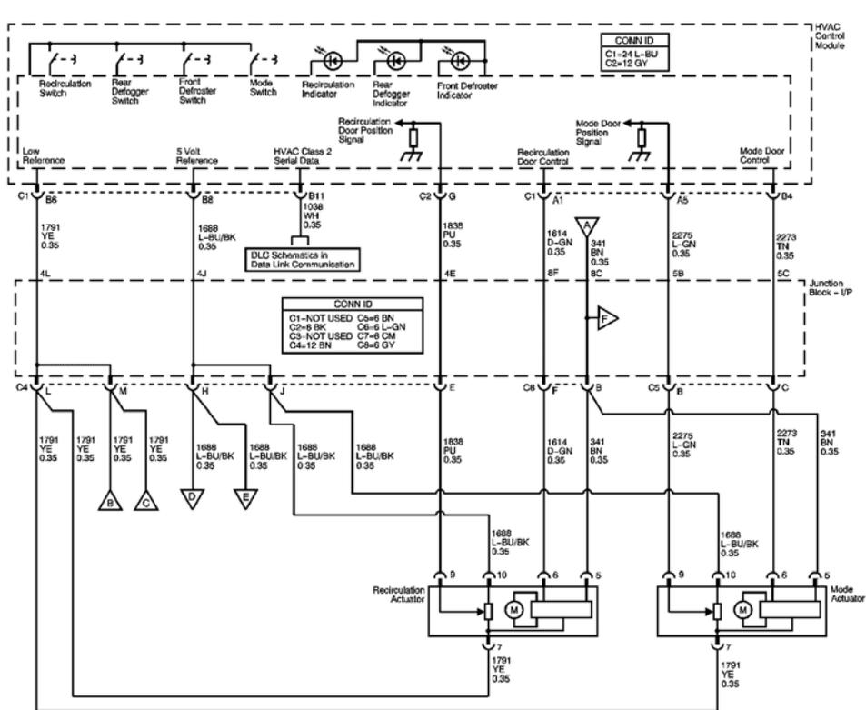
**Fig. 2: Mode and Recirculation Controls, Front Defrost and Rear Defog Controls Schematics**
