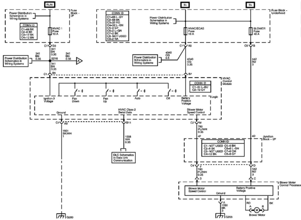
**Fig. 1: Power, Grounding, DLC, and Blower Control Schematics**
