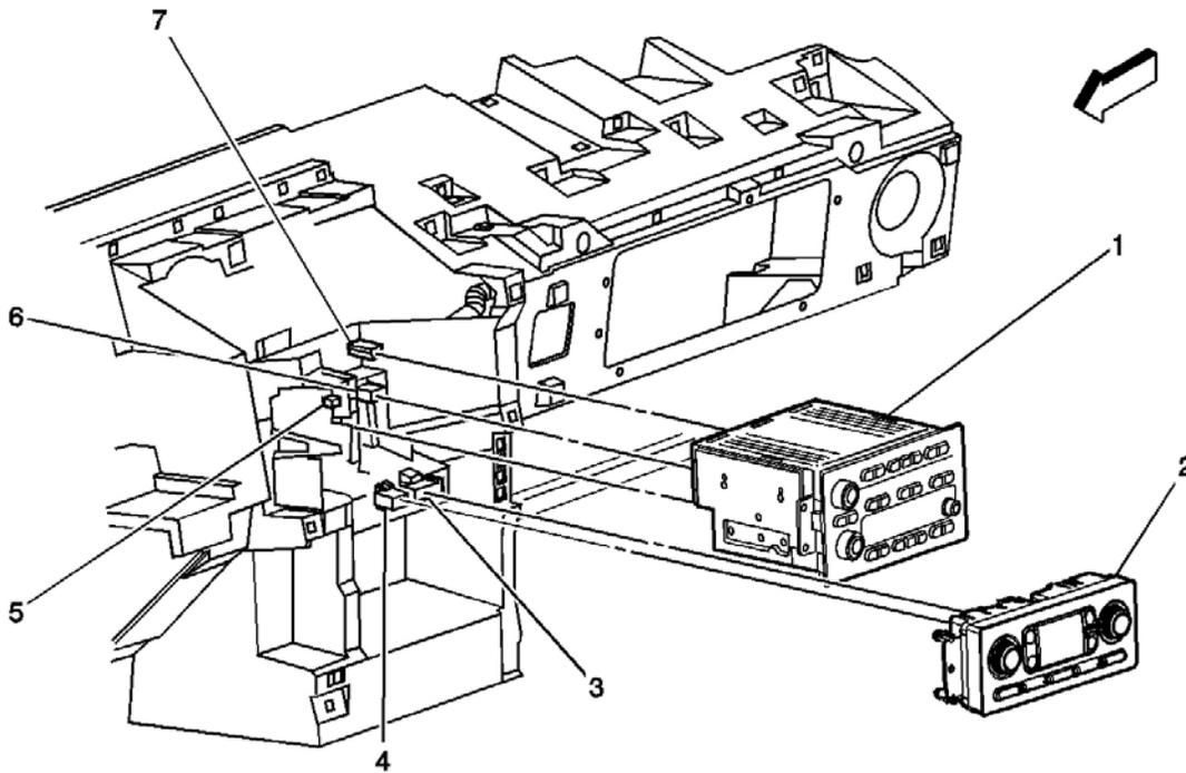
**Fig. 10: HVAC Control Module Component Views**
