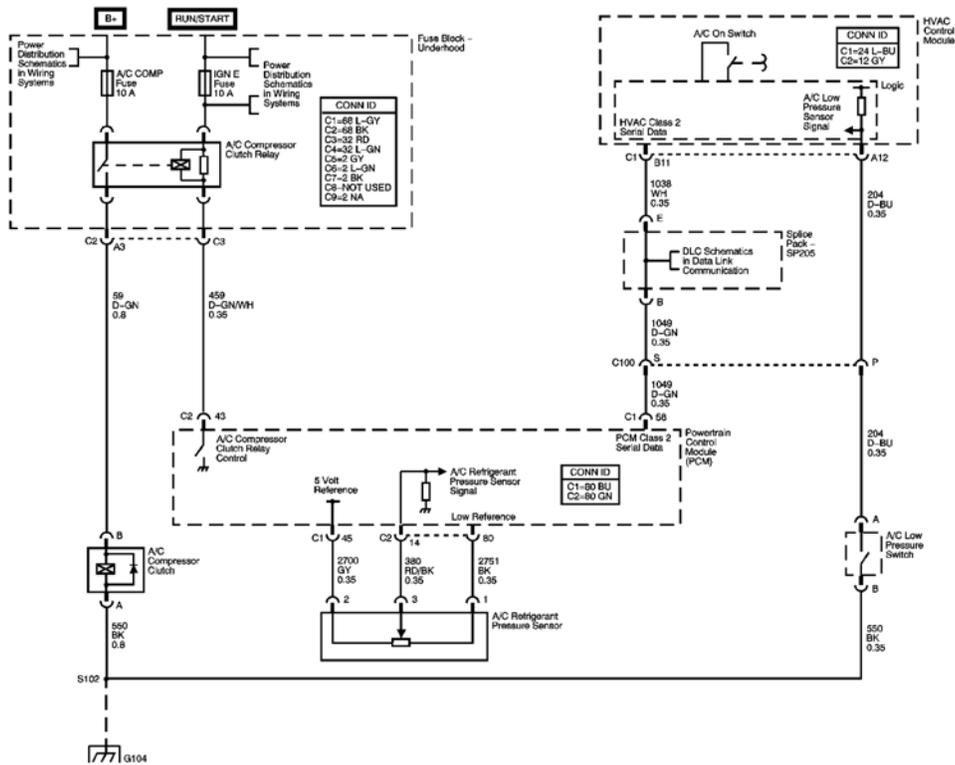
**Fig. 5: Air Conditioning Compressor Control Schematics**
