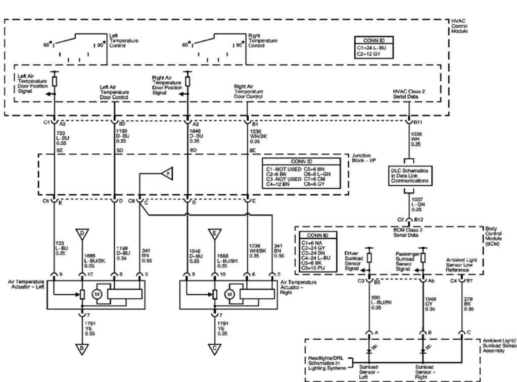
**Fig. 3: Temperature Controls and Sunload Sensors Schematics**
