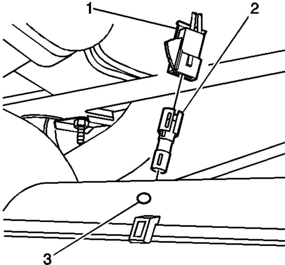
**Fig. 25: Upper Right Air Temperature Sensor & Air Distributor Duct**
