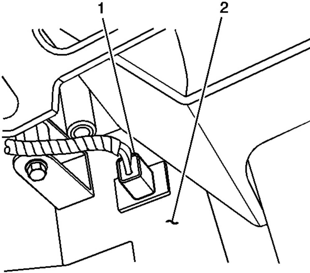
**Fig. 30: Lower Right Air Temperature Sensor & HVAC Module**
