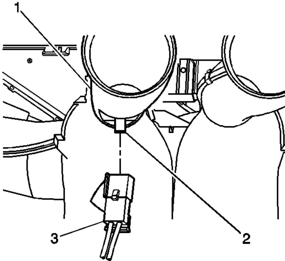
**Fig. 27: Upper Left Air Temperature Sensor & Air Distributor Duct**
