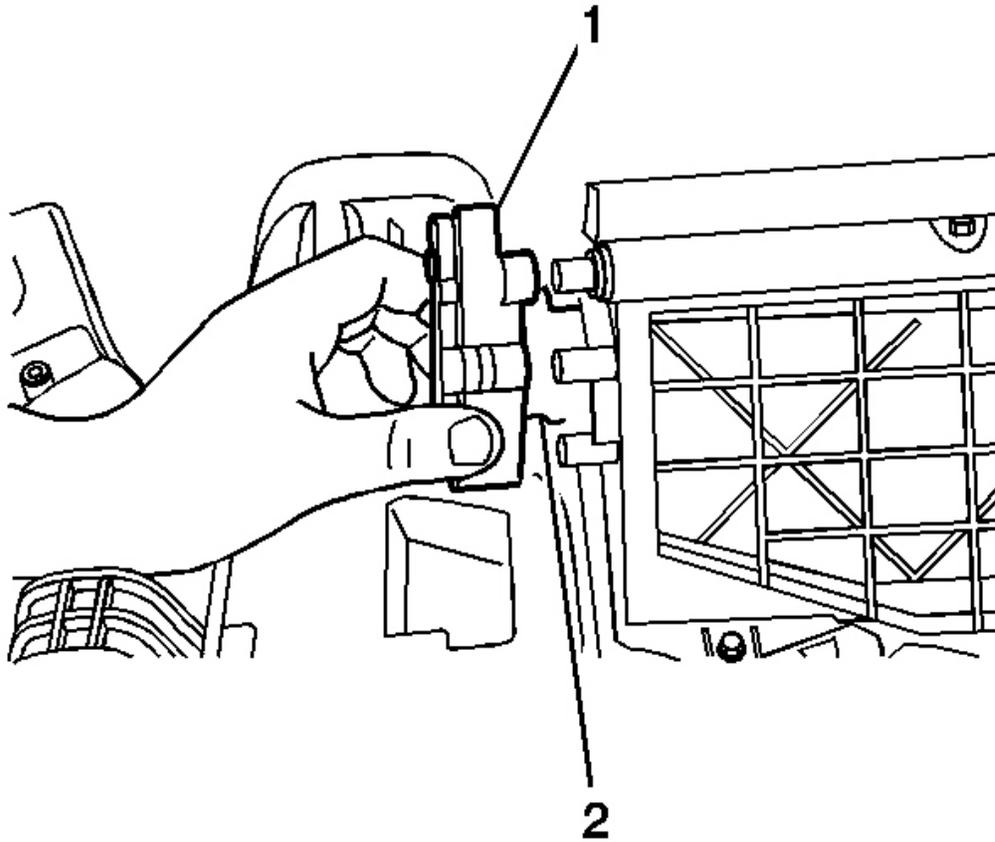
**Fig. 16: Recirculation Actuator & Recirculation Housing (Visteon)**
